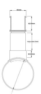
Grates longer than 1500mm supplied in sections. Tile Inserts longer than 1200mm supplied in sections. Channels over 3000mm supplied in sections with joiner. +/-2mm tolerance on dimensions.
