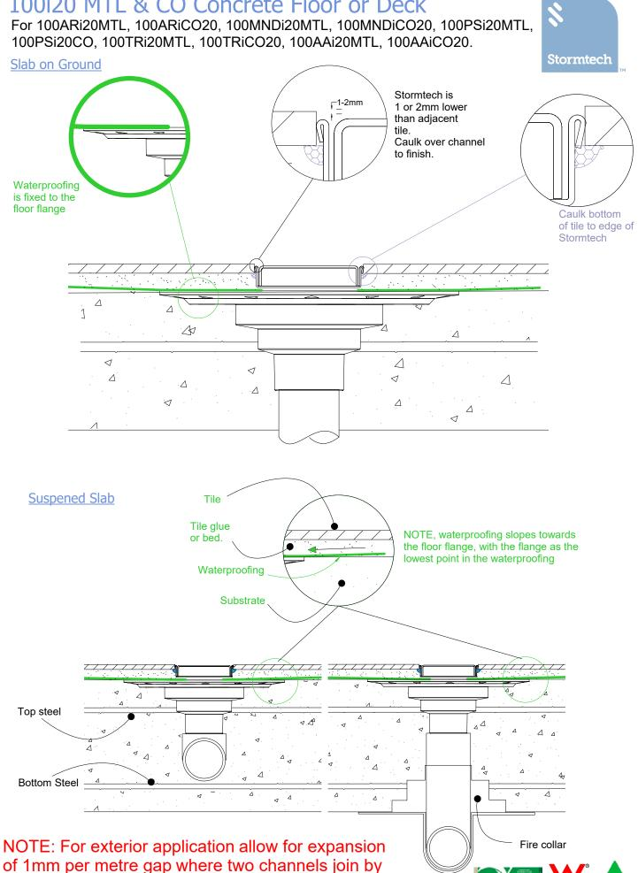
using quality suitable flexible sealant on channel joiners.
