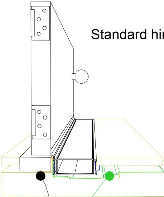
Aluminium angle to support waterproofing and junction between channel and door sil.
