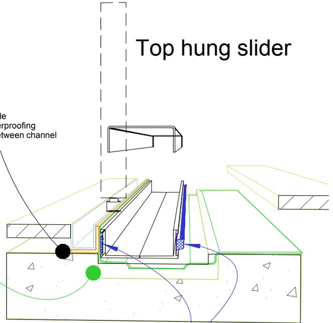
Aluminium angle to support waterproofing and junction between channel and door track.
