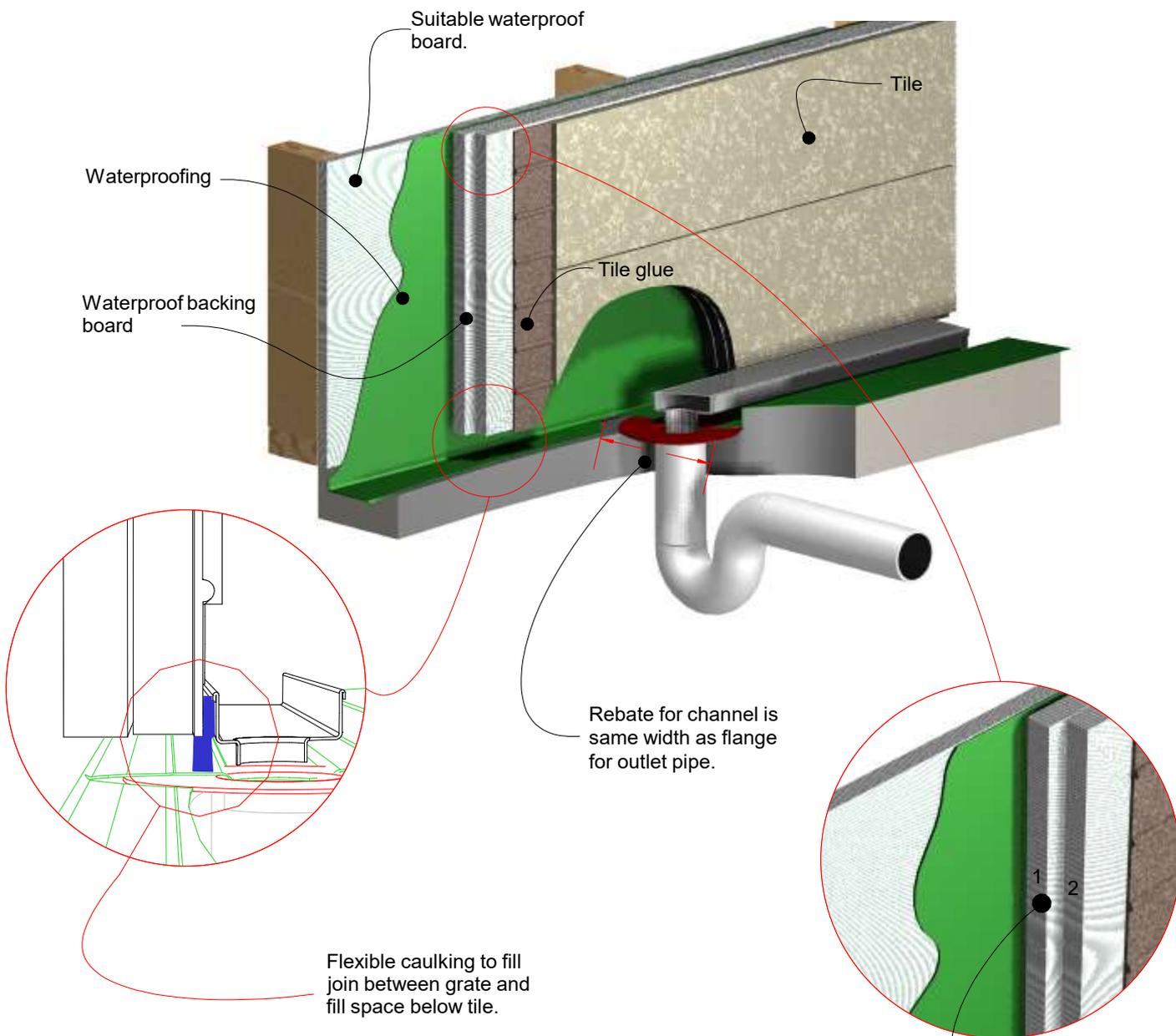
NOTE, due to the diameter of leak control or puddle flanges up to two layers of waterproof backing board or villa board may be needed to pack out wall before tiling.
