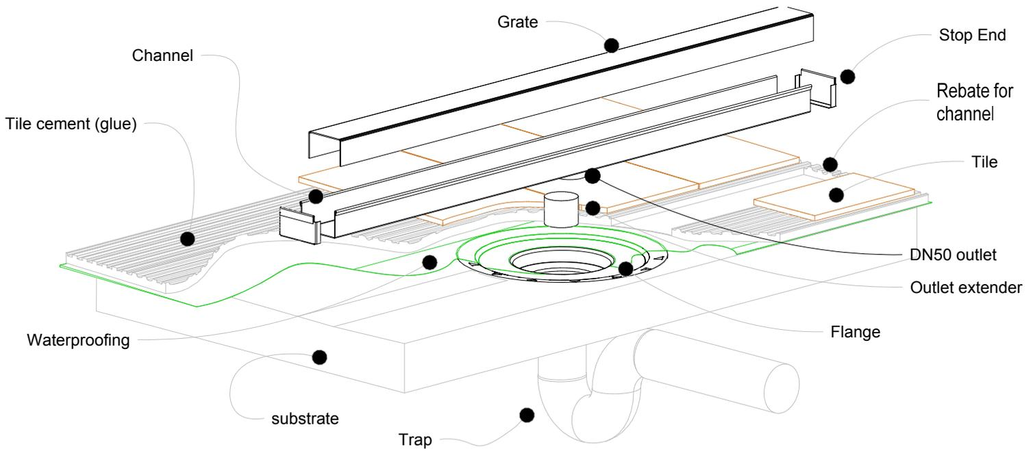
NOTE, this method requires the channel system to be ABOVE and SEPARATE from the WATERPROOFING.
